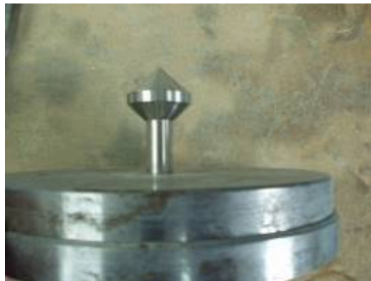
Graphic B.15: The second version of insert, with a conic form to facilitate the filling around the insert when coarse aggregates are used.
