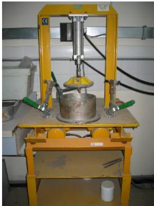
Graphic B.2: Vibration table and steel cylinder for the compaction of the granular sample
