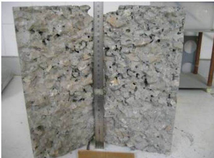
Graphic B.7: Pictures of the F5 mix after curing. Segregation is due to the gap graded skeleton. No cracks are visible.
