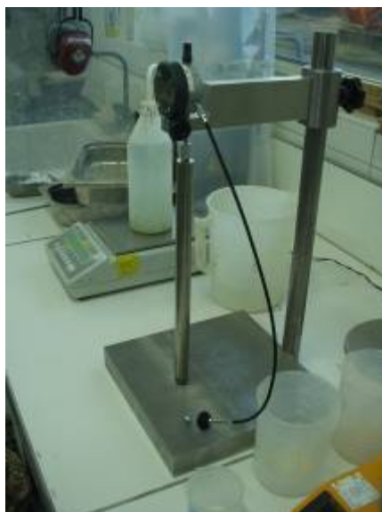
Graphic B.11: Tool realized for length measurement of Ø16x 32 cm of well graded aggregate. The zero is made thanks an invar bar. The contact with the inserts of the sample or the bar are ensured by two steel balls.
