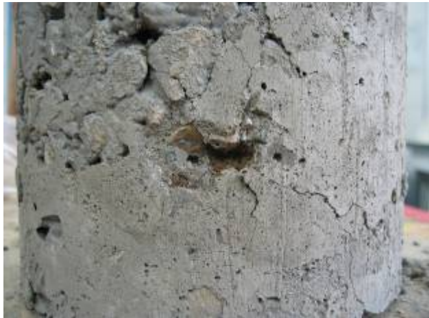
Graphic B.6: Pictures of the F1 mix after curing. Segregation is due to the gap graded skeleton. Cracks are visible as well as brown scaling due to quicklime hydration in slag particles
