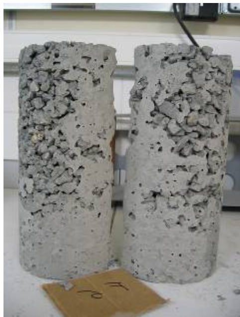
Graphic B.7: Pictures of the F5 mix after curing. Segregation is due to the gap graded skeleton. No cracks are visible.
