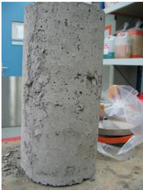
Graphic B.6: Pictures of the F1 mix after curing. Segregation is due to the gap graded skeleton. Cracks are visible as well as brown scaling due to quicklime hydration in slag particles
