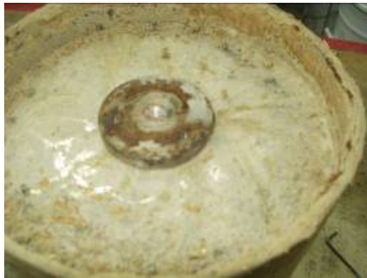
Graphic B.14: The insert after removal of the steel plate
