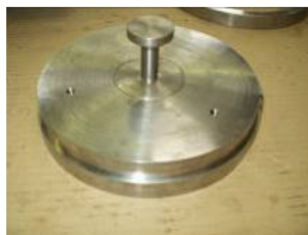
Graphic B.13: Detail of the steel plate (9) with the first version of insert (8)
