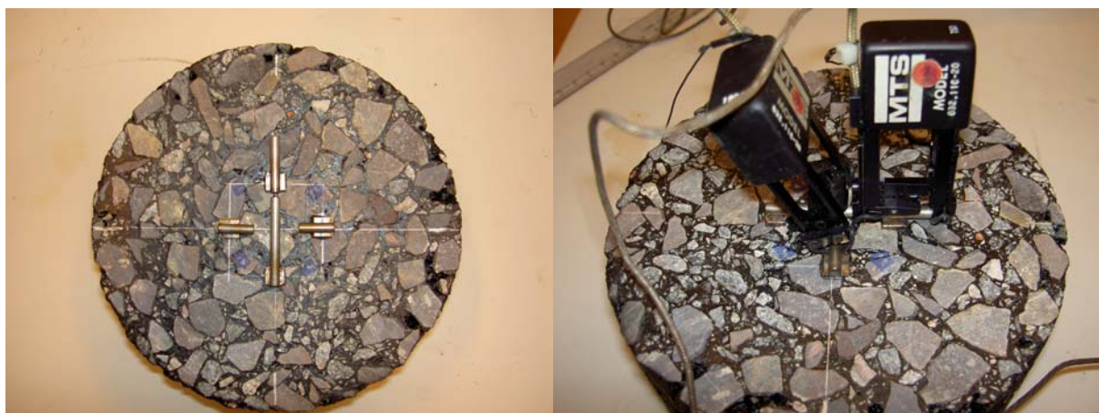
Figure 5: Mounting of strain gauges for measuring the complex modulus according to Kim et al [1].
