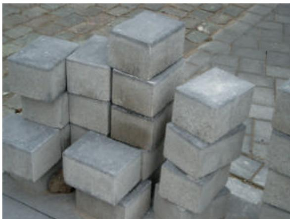
Photocatalytic pavement blocks, the  $\text{TiO}_2$  is added in the upper layer
